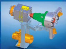
Cross extrusion head with hydraulic tool centering
