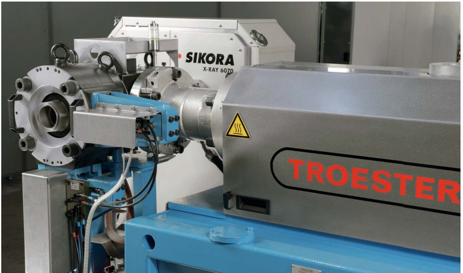
The new technology concept from TROESTER and SIKORA for quality assurance by automatic wall thickness centering
